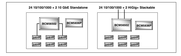
The BCM56502 is the fifth generation of the highly-integrated and cost-effective StrataSwitch and StrataXGS product line and is a single-chip solution with 24-GbE ports and two 10-GbE/HiGig+ uplink ports.
